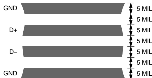
Figure 34. Typical Arrangement of Signal Tracks
