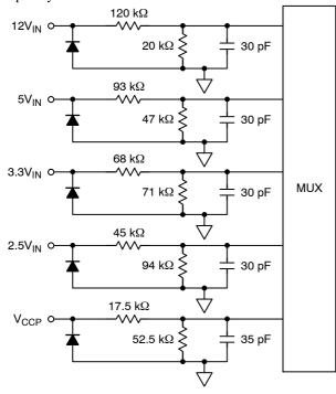
Figure 14. Internal Structure of Analog Inputs
