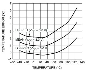
Figure 4. Local Temperature Error
