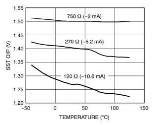
Figure 5. SST O/P Level vs. Temperature
