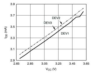
Figure 6. Supply Current vs. Voltage
