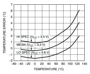
Figure 7. Remote Temperature Error
