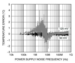
Figure 13. Remote Temperature Error vs. Power Supply Noise
