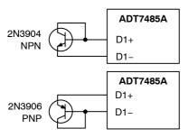
Figure 16. Connections for NPN and PNP Transistors
