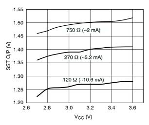
Figure 2. SST O/P Level vs. Supply Voltage
