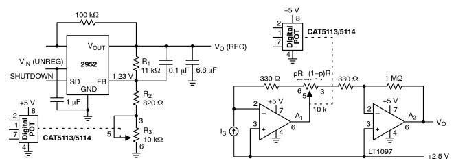
Figure 9. Programmable Voltage Regulator
