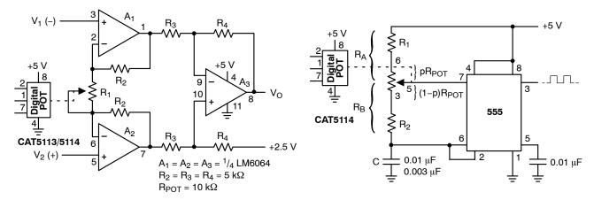
Figure 7. Programmable Instrumentation Amplifier
