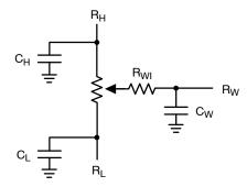
Figure 4. Potentiometer Equivalent Circuit
