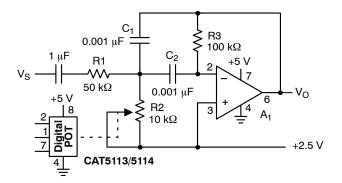
Figure 11. Programmable Bandpass Filter
