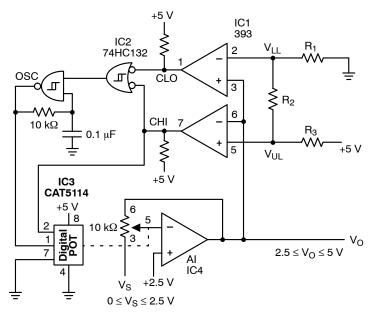
Figure 12. Automatic Gain Control
