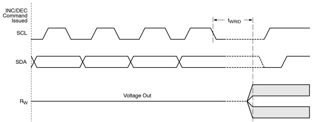
Figure 13. Increment/Decrement Timing Limits
