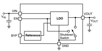
Figure 2. CAT6218 Functional Block Diagram
