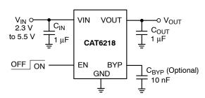
Figure 1. Typical Application Circuit
