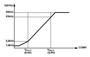
Figure 26. Frequency Reduction Curve in CV Mode
