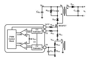
Figure 22. Simplified PSR Flyback Converter Circuit
