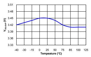
Figure 12. Gate Output Clamp Voltage (V<sub>CLAMP</sub>) vs. Temperature
