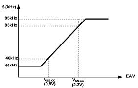
Figure 28. Frequency Reduction Curve in CC Mode
