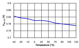
Figure 16. Starting Voltage of Frequency Decreasing of CC Regulation (V<sub>SN-CC</sub>) vs. Temperature Figure 17. Ending Voltage of Frequency Decreasing of CC Regulation (V<sub>SG-CC</sub>) vs. Temperature
