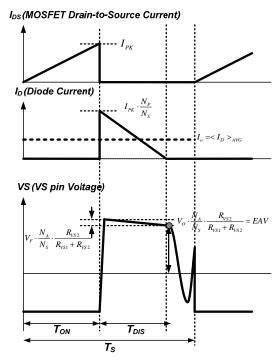
Figure 23. DCM Flyback Converter Waveforms
