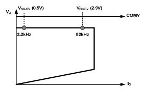
Figure 25. Frequency Reduction with COMV
