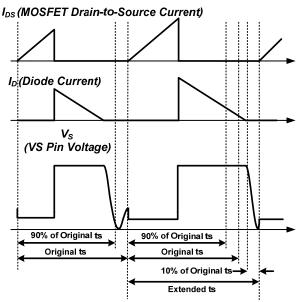
Figure 24. BCM Operation Function Waveform
