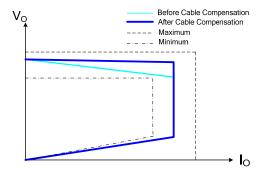
Figure 1. Typical Output V-I Characteristic
