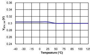
Figure 18. Threshold Voltage for Current Limit (V<sub>STH</sub>) vs. Temperature
