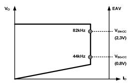
Figure 27. Frequency Reduction with EAV
