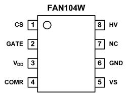
Figure 5. Pin Configuration
