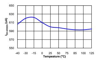
Figure 8. Operating Current (I<sub>DD-OP</sub>) vs. Temperature
