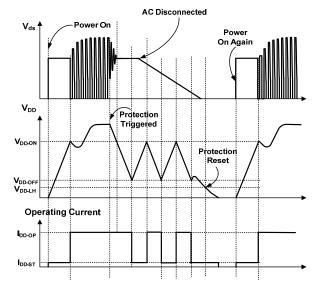
Figure 32. Latch-Mode Operation
