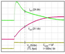
Figure 43. Quasi-Static Source Current with  $V_{DD}$  = 8 V (Note 14)
