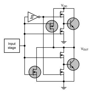
Figure 46. Miller Drive Output Architecture
