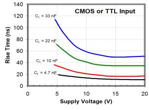
Figure 38. Rise Time vs. Supply Voltage
