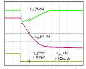
Figure 44. Quasi-Static Sink Current with V<sub>DD</sub> = 8 V (Note 14)
