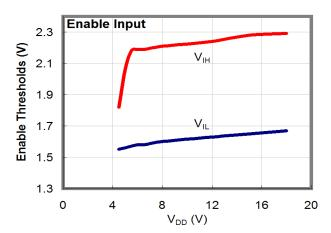
Figure 20. Input Thresholds % vs. Supply Voltage
