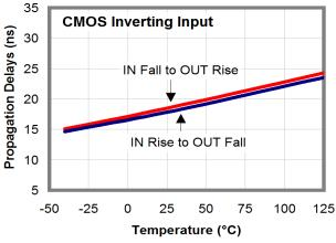
Figure 34. Propagation Delays vs. Temperature
