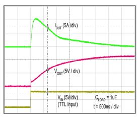
Figure 41. Quasi-Static Source Current with V<sub>DD</sub> = 12 V (Note 14)
