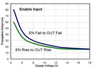
Figure 31. Propagation Delay vs. Supply Voltage
