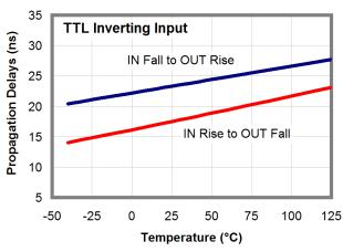
Figure 35. Propagation Delays vs. Temperature
