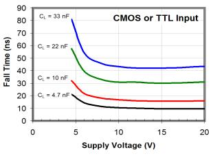
Figure 37. Fall Time vs. Supply Voltage
