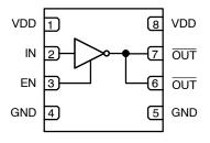
Figure 1. FAN3121 Pin Configuration
