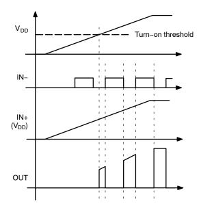
Figure 50. Inverting Startup Waveforms
