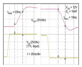
Figure 40. Rise / Fall Waveforms with 10 nF Load
