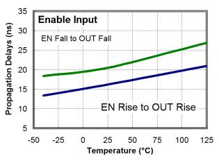
Figure 36. Propagation Delays vs. Temperature
