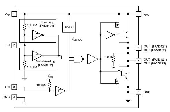
Figure 7. Block Diagram
