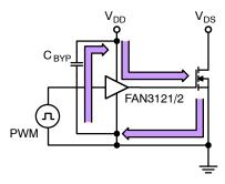
Figure 47. Current Path for MOSFET Turn-On
