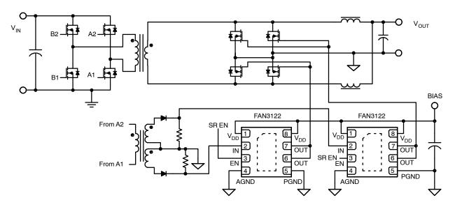
Figure 53. Full-Bridge Synchronous Rectification
