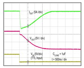
Figure 42. Quasi-Static Sink Current with V<sub>DD</sub> = 12 V (Note 14)
