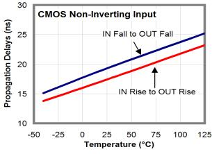
Figure 32. Propagation Delays vs. Temperature
