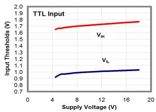
Figure 18. Input Thresholds vs. Supply Voltage
