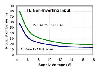
Figure 30. Propagation Delay vs. Supply Voltage
