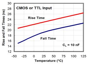
Figure 39. Rise and Fall Time vs. Temperature
