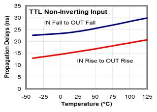
Figure 33. Propagation Delays vs. Temperature
