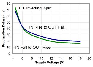
Figure 28. Propagation Delay vs. Supply Voltage
