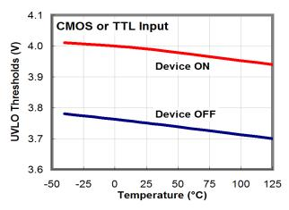
Figure 24. TTL Input Thresholds vs. Temperature
