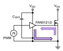
Figure 48. Current Path for MOSFET Turn-Off
