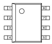
Figure 4. SOIC-8 (Top View)
