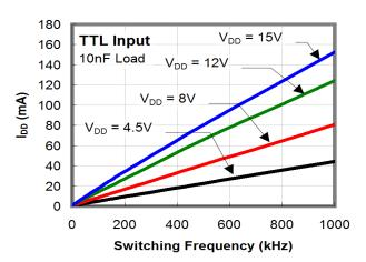
Figure 14.  $I_{DD}$  (10 nF Load) vs. Frequency
