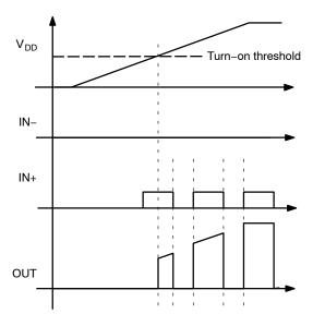
Figure 52. Non-Inverting Startup Waveforms
