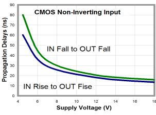
Figure 29. Propagation Delay vs. Supply Voltage
