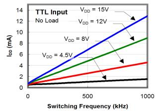
Figure 12. I<sub>DD</sub> (No-Load) vs. Frequency
