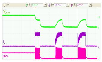
Figure 35. Over-Current Fault Response,  $R_{LOAD} = 1 \ \Omega, 50 \ \mu s/div.$
