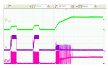
Figure 37. Overload Recovery to Light Load, 50 µs/div.
