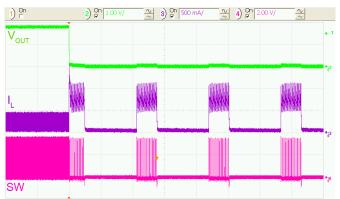
Figure 33. Metallic Short Applied at V<sub>OUT</sub>, 50 µs/div.
