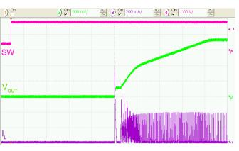
Figure 38. Soft-Start,  $R_{LOAD} = 50 \Omega$ , 20 µs/div.
