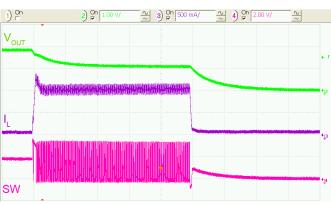
Figure 36. Over-Current Fault Response,  $R_{LOAD} = 1 \Omega$
