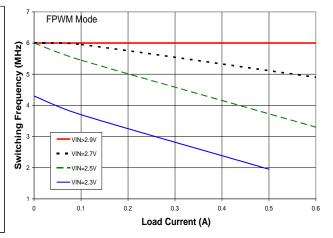
Figure 14. Effect of t<sub>OFF(MIN)</sub> on Reducing Switching Frequency
