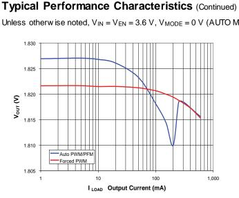
Figure 11. Load Regulation, Auto PFM / PWM and Forced PWM
