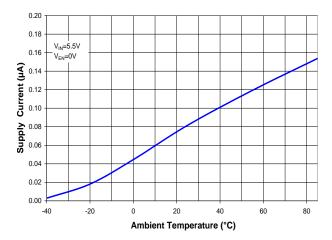
Figure 19. Shutdown Current vs. Temperature
