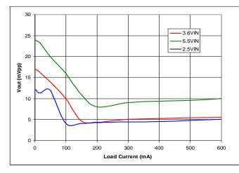
Figure 13. 1.233 V<sub>OUT</sub> Peak-to-Peak Output Voltage Ripple
