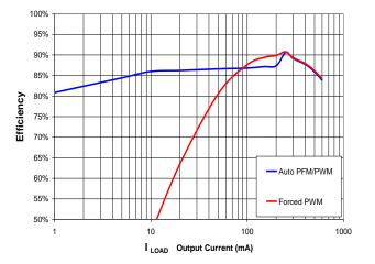
Figure 8. Efficiency, Auto PWM/PFM vs. Forced PWM
