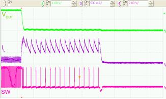
Figure 34. Metallic Short Applied at VOUT
