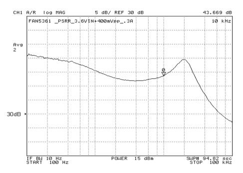
Figure 40. Power Supply Rejection Ratio at 300 mA Load
