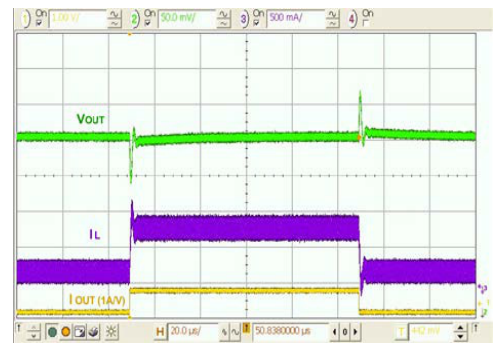
Figure 19. Load Transient, 200–800–200 mA, 100 ns Edge
