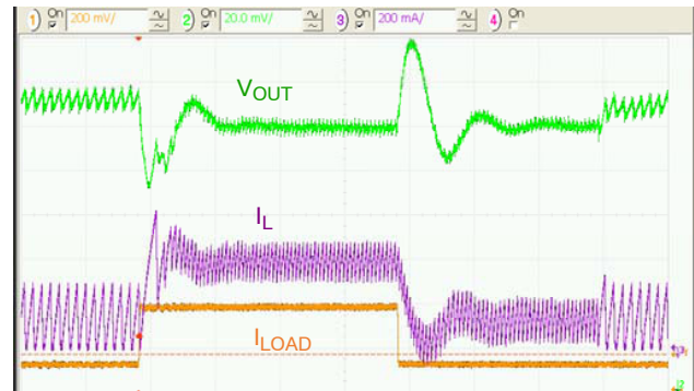
Figure 22. Load Transient 150 mA to 400 mA, V_{IN} = 3.6\text{ V} , t_{RISE} = t_{FALL} = 100\text{ ns} , 5 \mu\text{s} /div.
