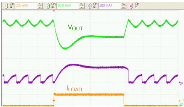
Figure 23. Load Transient 50 mA to 250 mA, V_{IN} = 3\text{ V} , t_{RISE} = t_{FALL} = 100\text{ ns} , 5\text{ }\mu\text{s/div} .
