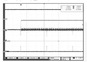
Figure 10. Mode Transition from 1x to 1.5x Mode,  $V_{\text{IN}}$ =3.6V ( $V_{\text{CATHODE}}$  Ramp Up)
