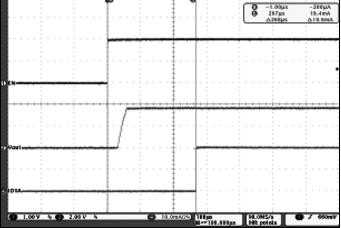
Figure 15. Soft-Start with EN, V<sub>IN</sub>=3.6V, I<sub>LEDx</sub>=20mA
