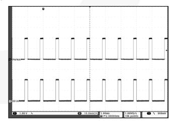
Figure 9. PWM Dimming V<sub>IN</sub>=3.6V, I<sub>LEDx</sub>=20mA, EN=1kHz with 20% Duty Cycle
