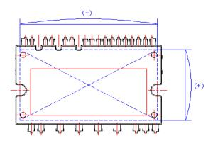
Figure 6. Flatness Measurement Position
