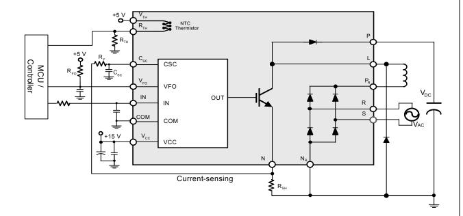
**Figure 9. Typical Application Circuit**
