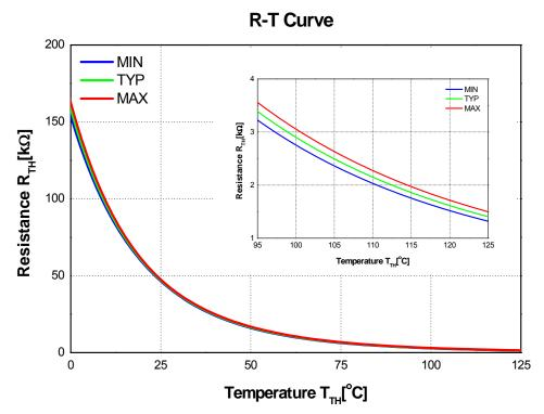
Figure 5. R-T Curve of The Built-in Thermistor
