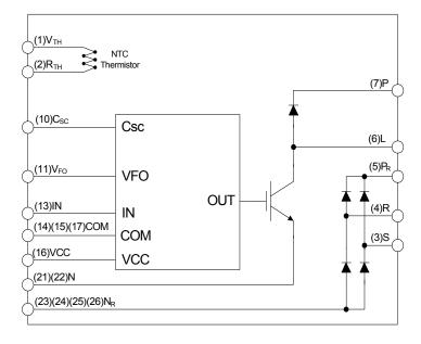
Figure 3. Internal Block Diagram
