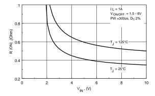
Figure 3. On-Resistance Variation with Input Voltage.
