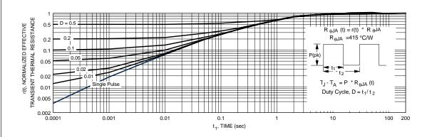
Figure 4. Transient Thermal Response Curve.
