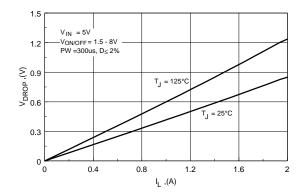
Figure 1. Conduction Voltage Drop Variation with Load Current.
