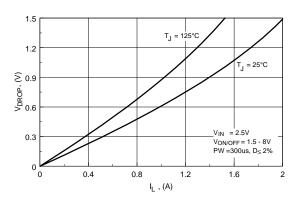
Figure 2. Conduction Voltage Drop
