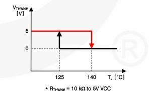
Figure 35. Gate Driver T<sub>J</sub> vs. V<sub>THWN#</sub>
