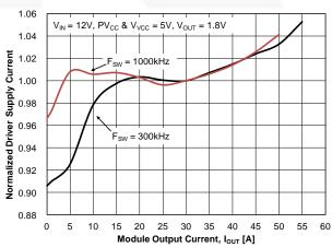
Figure 12. Driver Supply Current vs. Driver Supply Figure 13. Driver Supply Current vs. Output Current Voltage
