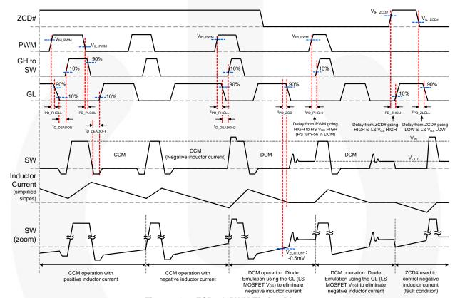
Figure 34. ZCD# & PWM Timing Diagram
