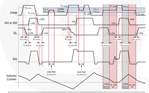
tpD\_XXX = propagation delay from external signal (PWM, ZCD#, etc.) to IC generated signal. Example : tpD\_PHGLL = PWM going HIGH to low-side MOSFET VGS (GL) going LOW t<sub>D\_XXXX</sub> = delay from IC generated signal to IC generated signal. Example : t<sub>D\_DEADON</sub> - low-side MOSFET V<sub>GS</sub> LOW to high-side MOSFET V<sub>GS</sub> HIGH
