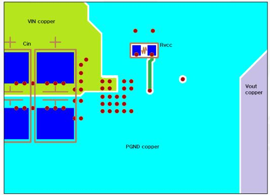
Figure 39. Single-Phase Board Layout Example – Bottom View (Mirrored)
