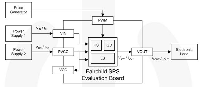
Figure 37. Power Loss and Efficiency Measurement Diagram
