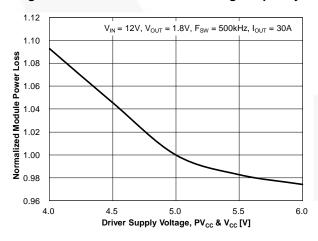
Figure 7. Power Loss vs. Input Voltage
