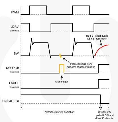
Figure 36. Catastrophic Fault Waveform
