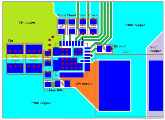
Figure 38. Single-Phase Board Layout Example – Top View
