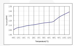
Figure 16. Start Timer (V<sub>FB</sub><V<sub>G</sub>)
