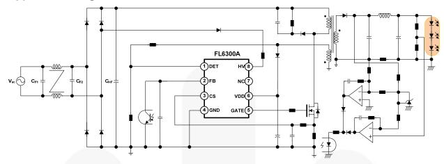
Figure 1. Typical Application Circuit for Flyback Converter
