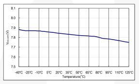
Figure 7. Turn-Off Threshold Voltage
