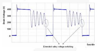
Figure 20. QR Operation in Extended Valley Voltage Detection Mode
