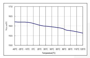
Figure 5. Turn-On Threshold Voltage
