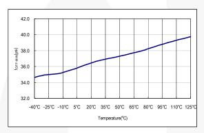
Figure 15. Minimum Off Time (V<sub>FB</sub>=V<sub>G</sub>)
