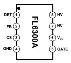
Figure 4. Pin Assignments
