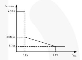
Figure 19. V<sub>FB</sub> vs. t<sub>OFF-MIN</sub> Curve
