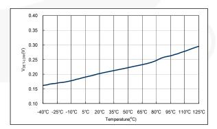
Figure 12. Lower Clamp Voltage
