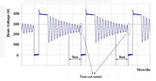
Figure 21. Internal t<sub>TIME-OUT</sub> Initiates New Cycle After Failure to Detect Valley Voltage
