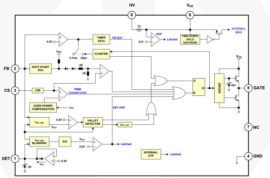
Figure 2. Functional Block Diagram
