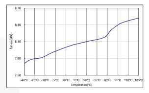
Figure 14. Minimum Off Time (V<sub>FB</sub>>V<sub>N</sub>)
