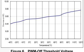
Figure 6. PWM-Off Threshold Voltage
