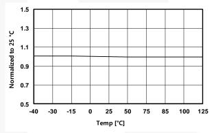
Figure 8. V<sub>OVP</sub> vs. Temperature
