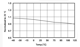
Figure 10. f<sub>MIN\_CC</sub> vs. Temperature
