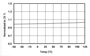
Figure 11. V<sub>CCR</sub> vs. Temperature
