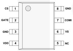
Figure 4. Pin Configuration (Top View)
