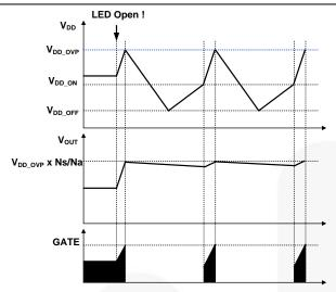
Figure 22. Waveforms in Open-LED Condition
