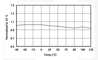
Figure 7. I<sub>DD-OP</sub> vs. Temperature
