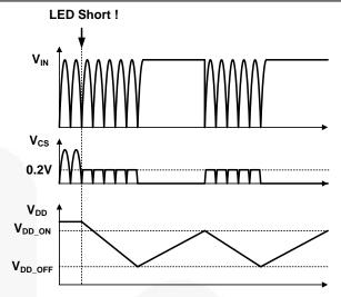
Figure 20. Waveforms in Short-LED Condition
