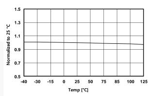
Figure 6. V<sub>DD-OFF</sub> vs. Temperature
