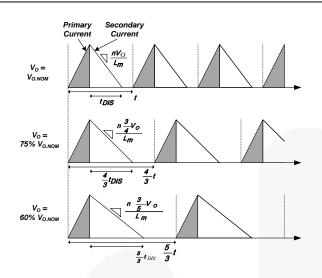
Figure 18. Primary and Secondary Current
