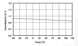
Figure 5. V<sub>DD-ON</sub> vs. Temperature
