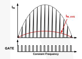
Figure 16. Input Current and Switching
