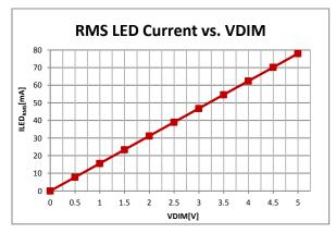
Figure 15. Current vs.  $V_{DIM}$  (Simulation results:  $R_{CS}$ =10  $\Omega$  /  $V_{AC}$  = 120 V)
