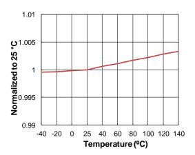
Figure 8. I<sub>LED2</sub> vs. Temperature
