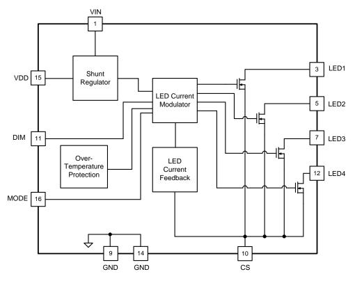
Figure 4. Simplified Block Diagram
