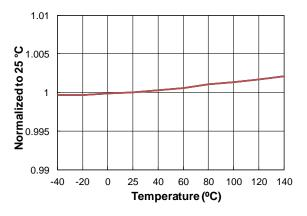
Figure 9.  $I_{LED3}$  vs. Temperature
