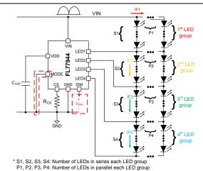
Figure 13. Analog or PWM dimming Application
