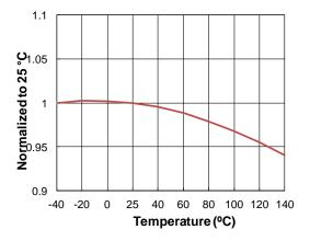
Figure 5. I<sub>QUIES.VIN</sub> vs. Temperature
