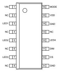
Figure 3. SOIC-16 EP (Top View)
