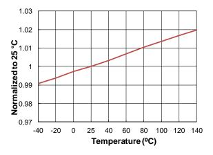
Figure 6. V<sub>DD</sub> vs. Temperature
