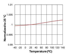
Figure 10. I<sub>LED4</sub> vs. Temperature
