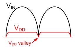
Figure 12.  $V_{DD}$  Ripple without  $C_{VDD}$
