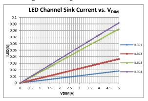
Figure 14. Measured LED Channel Sink Current vs.  $V_{DIM}$  (R<sub>CS</sub> = 10  $\Omega$ )
