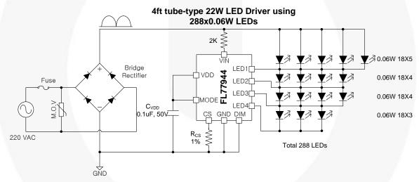
Figure 2. 22 W at 220 V<sub>AC</sub> LED Tube-Type Application
