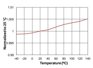
Figure 7. I<sub>LED1</sub> vs. Temperature
