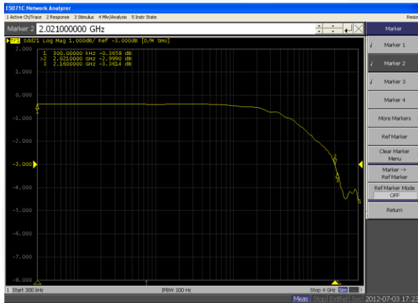
Figure 17. MHL Path SDD21 Insertion Loss Curve
