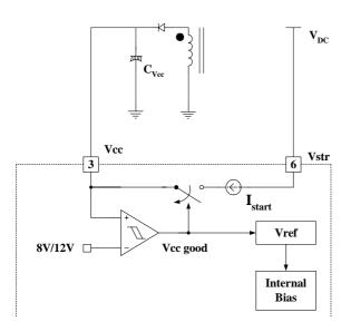
Figure 4. Internal startup circuit
