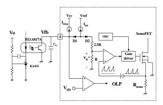
Figure 5. Pulse width modulation (PWM) circuit
