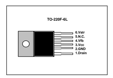
Figure 3. Pin Configuration (Top View)
