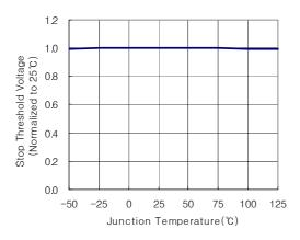
Stop Threshold Voltage vs. Temp
