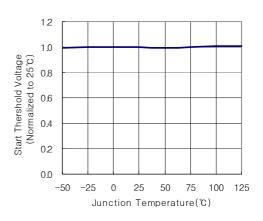
Start Threshold Voltage vs. Temp
