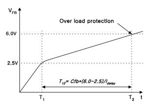
Figure 7. Over load protection
