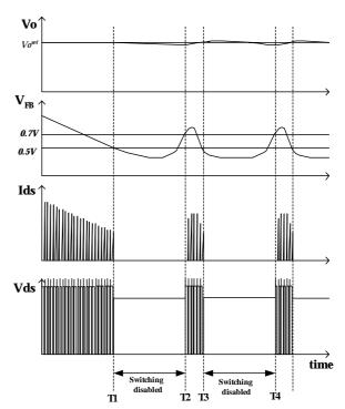
Figure 9. Waveforms of burst operation
