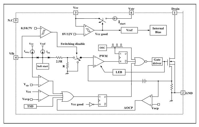
Figure 2. Functional Block Diagram of FSDM07652R
