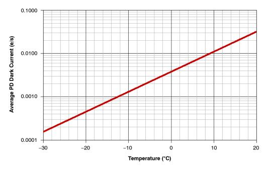
Figure 30. Photodiode Dark Current vs. Temperature
