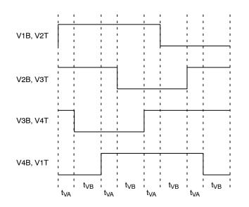
Figure 37. Line Timing L2. VCCD Line Timing to Transfer One Line of Charge from VCCD to the HCCD when Using All Four Outputs in Quad Mode
