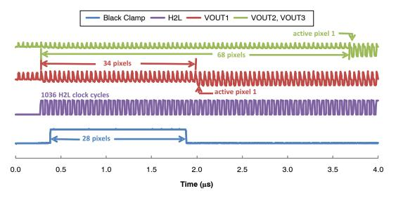
Figure 32. Video Output at Each Line Start
