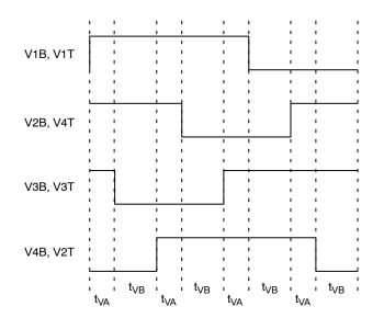
Figure 36. Line Timing L1. VCCD Line Timing to Transfer One Line of Charge from VCCD to the HCCD when Using the Bottom HCCD, Outputs A or B in Single or Dual Output Modes
