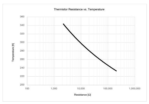
Figure 43. PGA with Integrated TEC, Thermistor Resistance vs. Temperature
