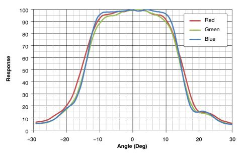
Figure 9. Color with Microlens Angle Response
