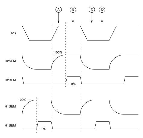
Figure 20. The Timing Diagram for Charge Multiplication
