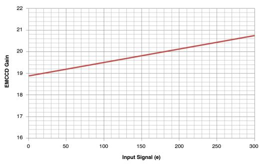
NOTE: The EMCCD voltage was set to provide 20x gain with an input of 180 electrons.
