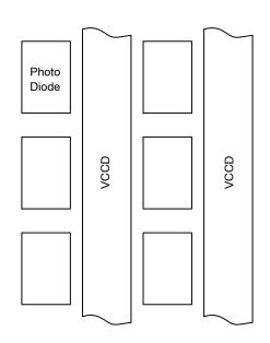
Figure 15. Illustration of 2 Columns and 3 Rows of Pixels
