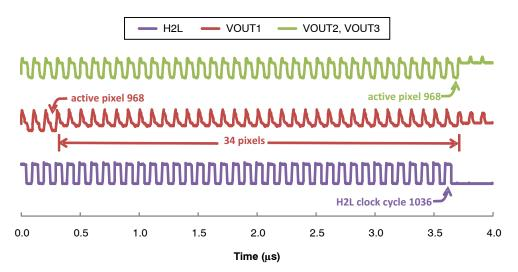
Figure 33. Video Output at End of Each Line for Dual or Quad Output Modes
