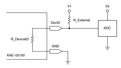
Figure 14. Device Identification Recommended Circuit
