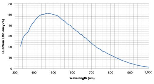
Figure 6. Monochrome QE with Microlens
