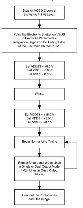
Figure 41. Timing Flow Chart for Long Integration Time
