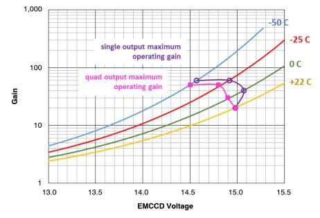
WARNING: The EMCCD should not be operated near saturation for an extended period, as this may result in gain aging and permanently reduce the gain. It should be noted that device degradation associated with gain aging is not covered under the device warranty.
