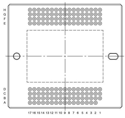
Figure 4. PGA Package Designations (Bottom View)
