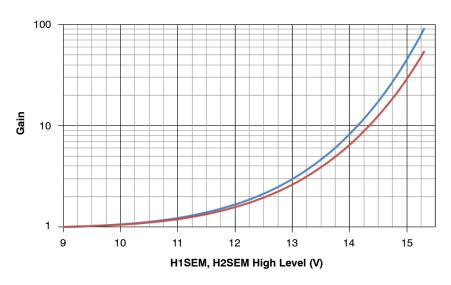
Figure 24. An Example Showing How Two Image Sensors Can Have Different Gain vs. Voltage Curves
