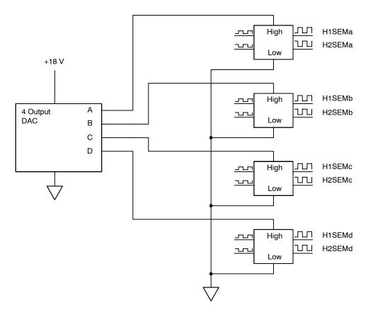
Figure 12. EMCCD Clock Adjustable Levels
