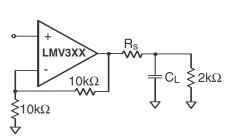
Figure 2. Typical Topology for driving a capacitive load
