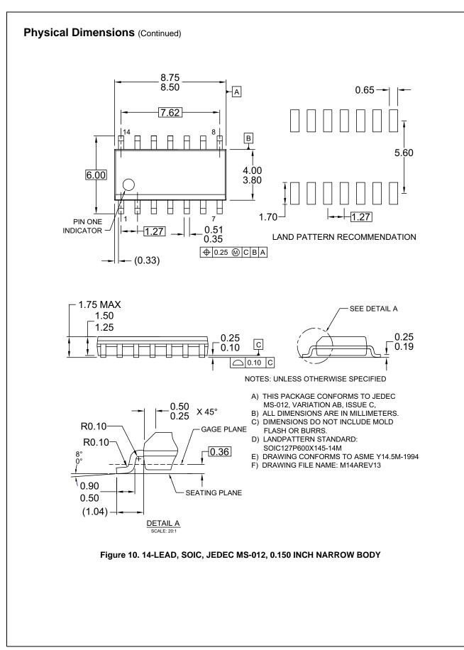
LMV321 / LMV358 / LMV324 — General-Purpose, Low Voltage, Rail-to-Rail Output Amplifiers
