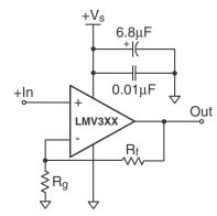
Figure 1. Typical Non-inverting configuration
