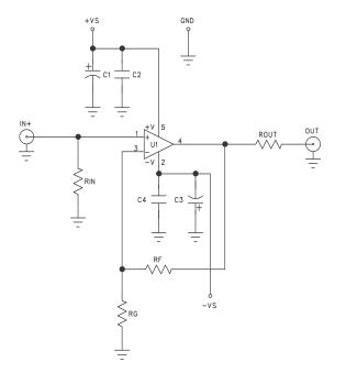
Figure 4b. LMV321 KEB014 schematic
