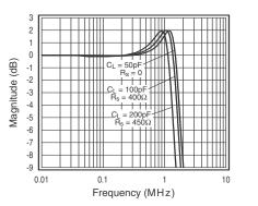
Figure 3. Frequency Response vs. C<sub>L</sub> for unity gain configuration
