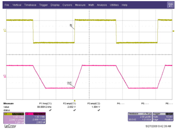
Figure 10. Non-Inverting Large Signal Step Response
