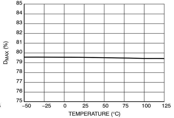
Figure 12. Maximum Duty Cycle  $D_{MAX}$
