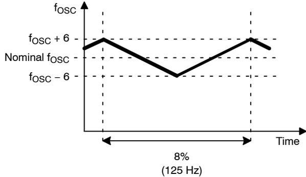
**Figure 30. Frequency Jittering**
