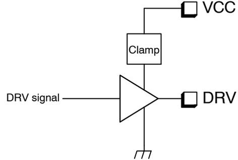
**Figure 31. Clamped Driver**
