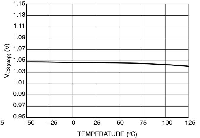
Figure 6. Threshold for Immediate Fault Protection Activation
