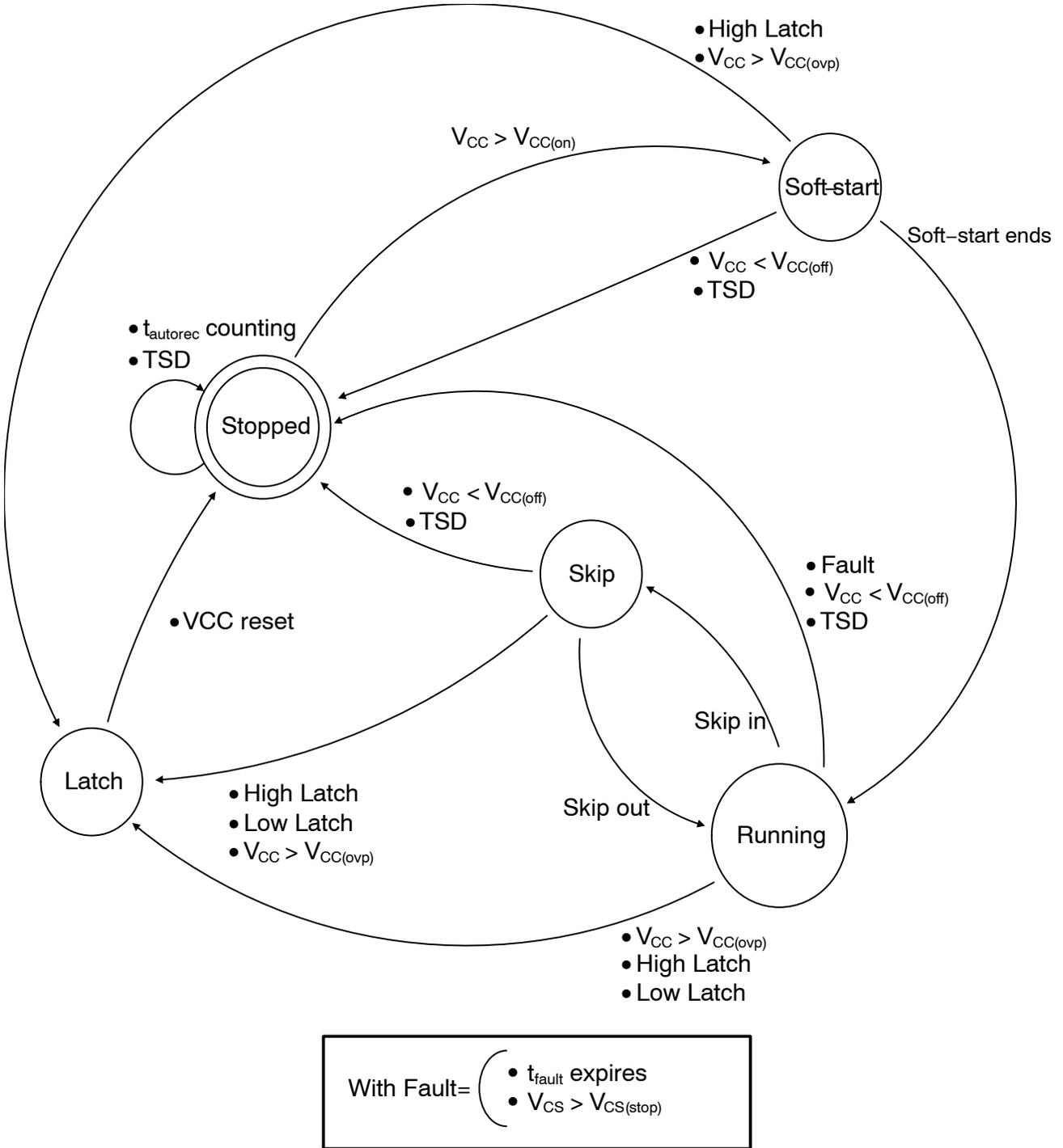
Figure 50. Controller Operation State Diagram (Autorecovery Protection)
