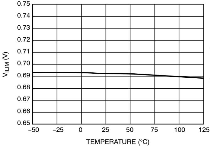
Figure 5. Maximum Internal Current Setpoint
