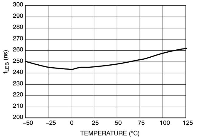
Figure 8. Leading Edge Blanking Duration t<sub>LEB</sub>
