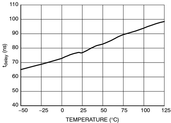
Figure 7. Propagation Delay t<sub>delay</sub>
