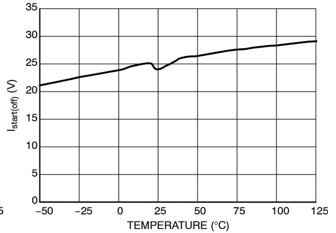
Figure 4. Off-State Leakage Current I<sub>start(off)</sub>
