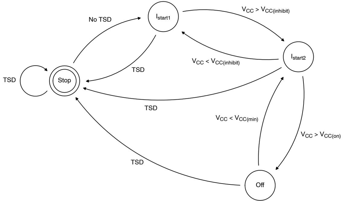
Figure 48. HV Start-up Current Source State Diagram
