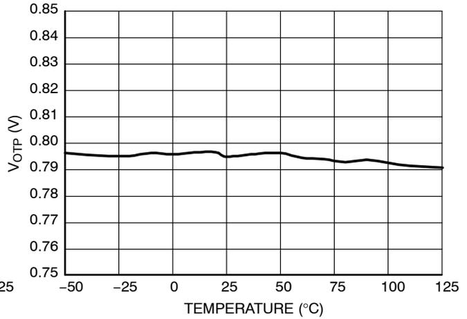
Figure 22. Latch Pin Low Threshold  $V_{OTP}$
