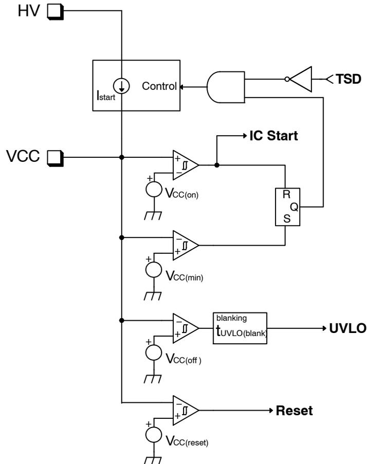
Figure 27. HV Start-up Current Source Functional Schematic
