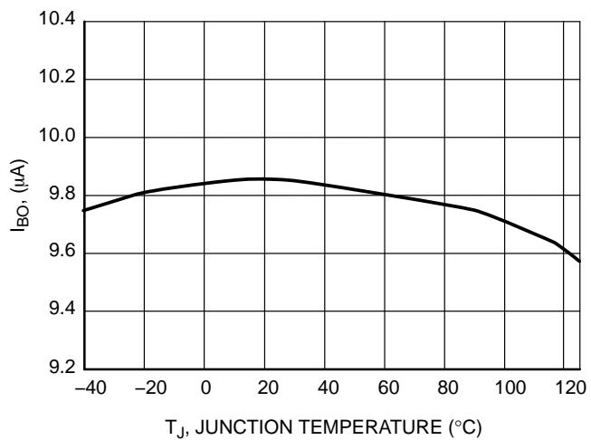
Figure 25.  $I_{B0}$  vs. Junction Temperature
