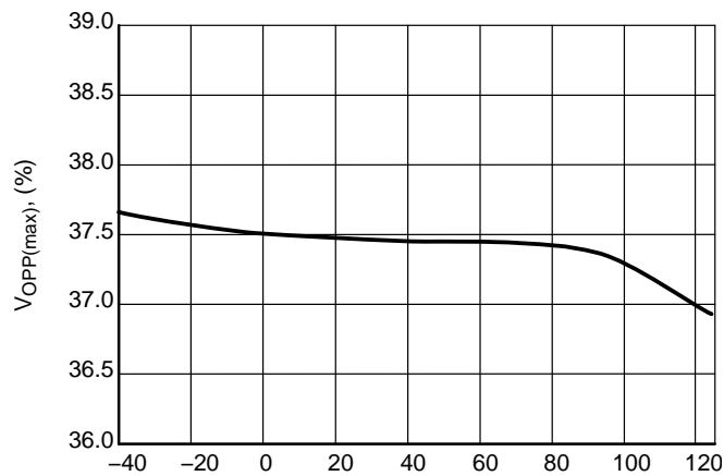
Figure 14.  $V_{OOPP(max)}$  vs. Junction Temperature
