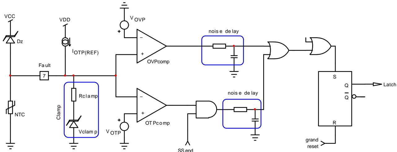
Figure 41. OVP/OTP Circuitry
