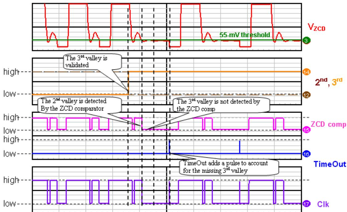
Figure 34. Time Out Case n°1: the 3<sup>rd</sup> Valley is Missing
