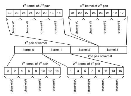
Figure 23. M1–SM: Data Output Order when Subsampling is Disabled
