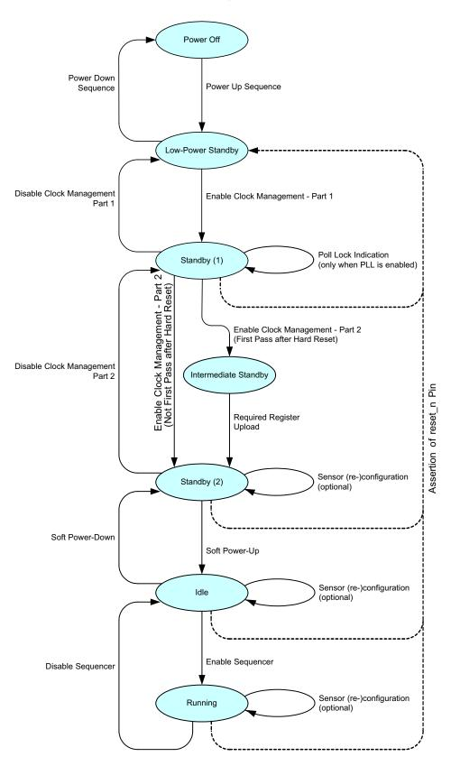
Figure 6. Sensor Operation Flowchart
