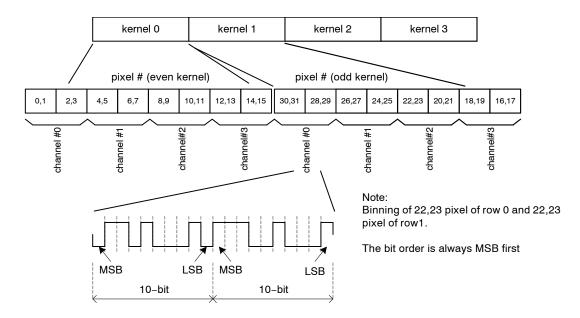
Figure 27. M1–SM: Data Output Order for 2 x 2 Binning
