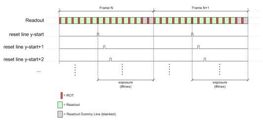
Figure 12. Integration Control in Rolling Shutter Mode
