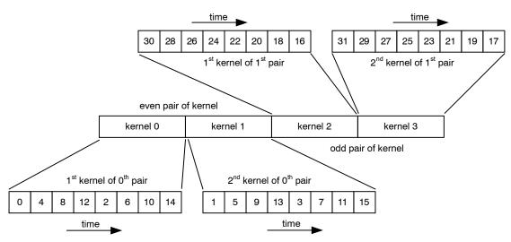
Figure 30. M2–SM: Data Output Order without Subsampling
