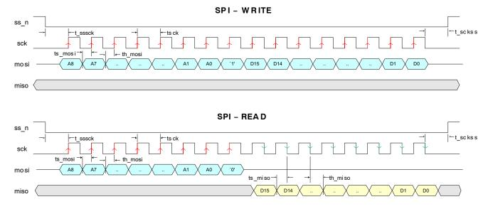
Figure 11. SPI Read and Write Timing Diagram
