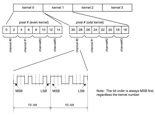
Figure 24. M1–SM: Data Output Order for Read–1–Skip–1 Subsampling
