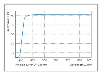
Figure 36. Transmission Characteristics of the Glass Lid
