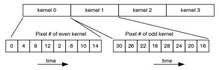
Figure 31. M2-SM: Data Output Order with Read-1-Skip-1 Subsampling
