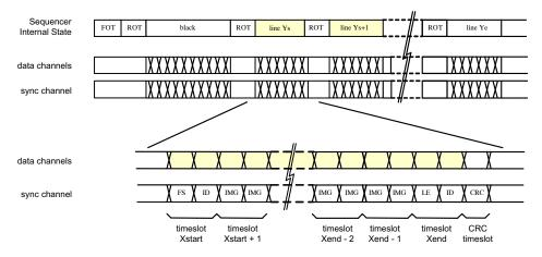
Figure 20 shows the details of the readout of a number of lines for single window readout, at the beginning of the frame.
