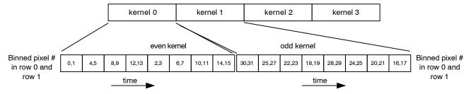
Figure 33. M2–SM: Data Output Order for 2 x 2 Binning
