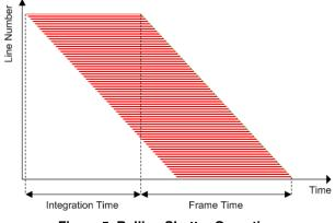
Figure 5. Rolling Shutter Operation
