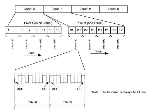
Figure 26. M1–SM: Data Output Order for Odd Pixels of Line During Checkerboard Subsampling
