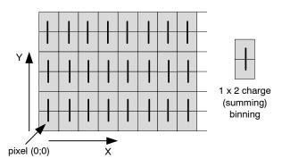
Figure 17. 1 x 2 Binning Scheme
