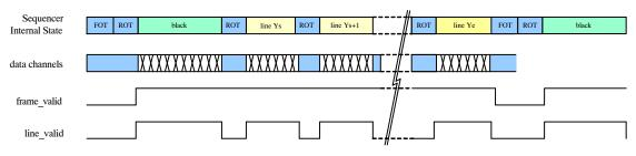
Figure 28. M2–SM: Frame Timing Indication
