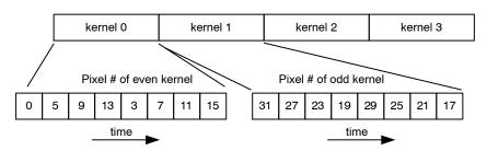
Figure 32. M2–SM: Data Output Order for Odd Pixel during Checkerboard Subsampling
