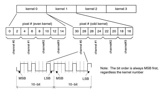
Figure 25. M1-SM: Data Output Order for Even Pixels of Line During Checkerboard Subsampling
