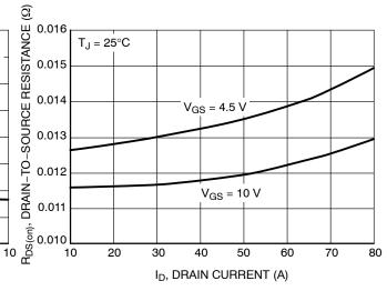
Figure 3. On-Resistance vs. Gate Voltage
