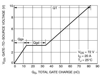
Figure 8. Gate-to-Source Voltage vs. Total Charge
