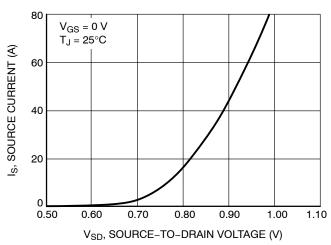
Figure 10. Diode Forward Voltage vs. Current
