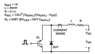
FIGURE 10. AVALANCHE ENERGY TEST CIRCUIT
