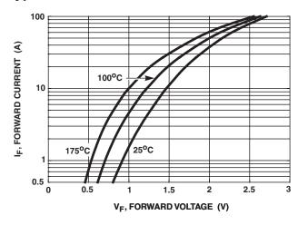
FIGURE 1. FORWARD CURRENT vs FORWARD VOLTAGE
