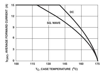
FIGURE 6. CURRENT DERATING CURVE
