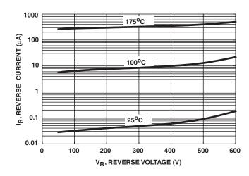
FIGURE 2. REVERSE CURRENT vs REVERSE VOLTAGE
