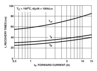
FIGURE 4. T<sub>rr</sub>, t<sub>a</sub> AND t<sub>b</sub> CURVES vs FORWARD CURRENT
