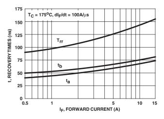
FIGURE 5. T<sub>rr</sub>, t<sub>a</sub> AND t<sub>b</sub> CURVES vs FORWARD CURRENT
