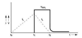
FIGURE 11. AVALANCHE CURRENT AND VOLTAGE WAVEFORMS
