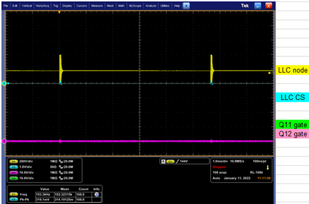
Figure 22. LCC at No Load
