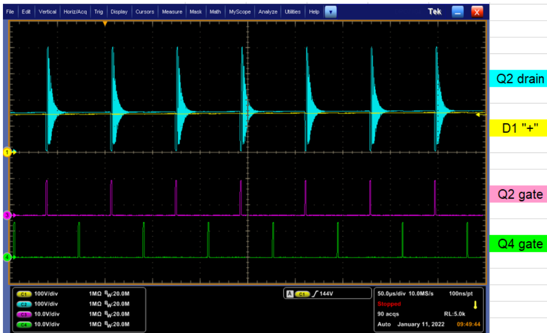
Figure 15. PFC Waveforms at No Load
