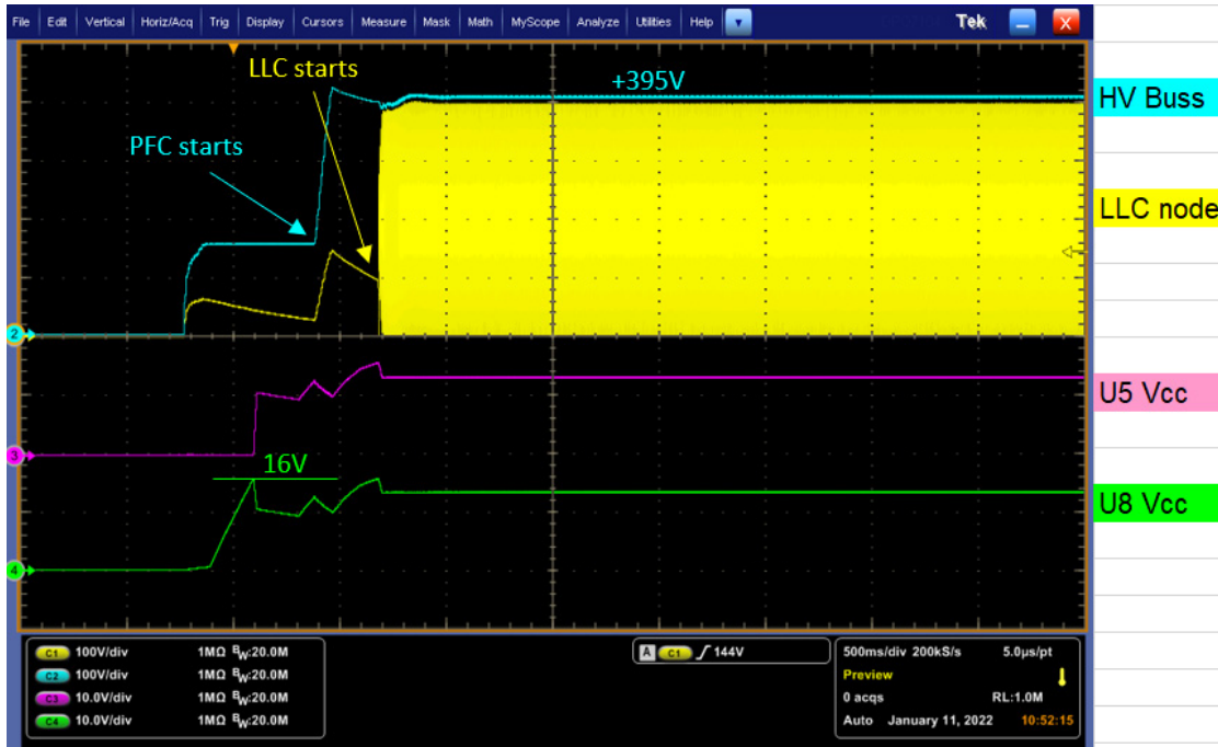
Figure 18. Power Supply Start-up Sequence
