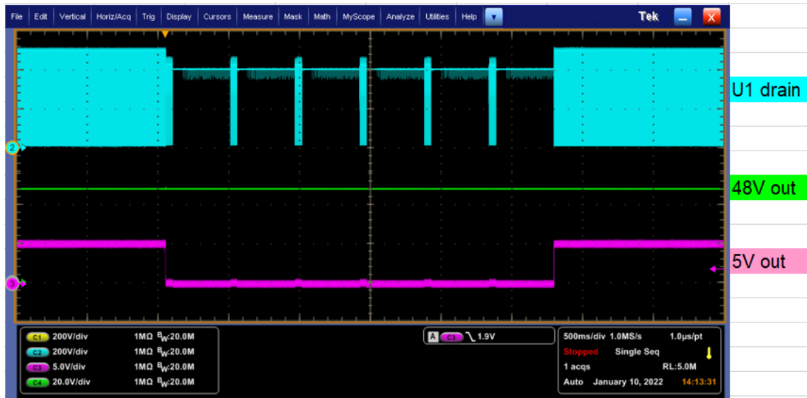
Figure 29. Shorting the 5 V Output
