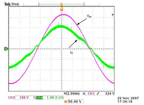
Figure 8.  $V_{ac}$  = 230 Vac,  $P_{in}$  = 309 W,  $V_{out}$  = 393 V,  $I_{out}$  = 0.77 A, PF = 0.996, THD = 6.1%
