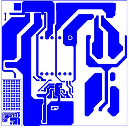
Figure 4. PCB Layout (Solder Side)
