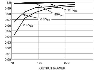
Figure 6. Power Factor vs. Output Power
