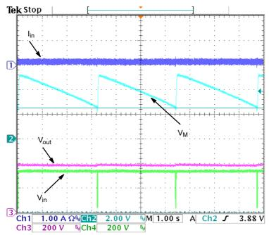
Figure 9.  $V_{ac}$  = 230 Vac,  $P_{in}$  = 147 mW,  $V_{out}$  = 396 V,  $I_{out}$  = 0 A
