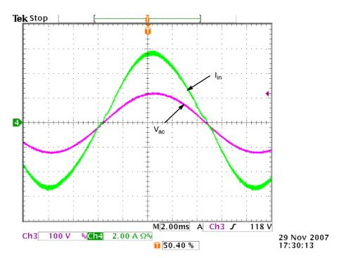
Figure 7.  $V_{ac}$  = 85 Vac,  $P_{in}$  = 326.5 W,  $V_{out}$  = 392.6 V,  $I_{out}$  = 0.77 A, PF = 0.999, THD = 3.74%
