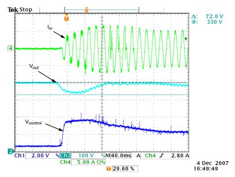
Figure 11.  $V_{ac}$  = 85 Vac,  $V_{out}$  = 392.6 V,  $I_{out}$  = 0 A ~ 0.77 A
