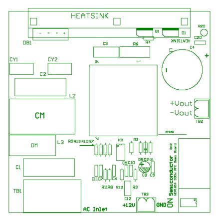
Figure 3. Components Placement (Component Side)
