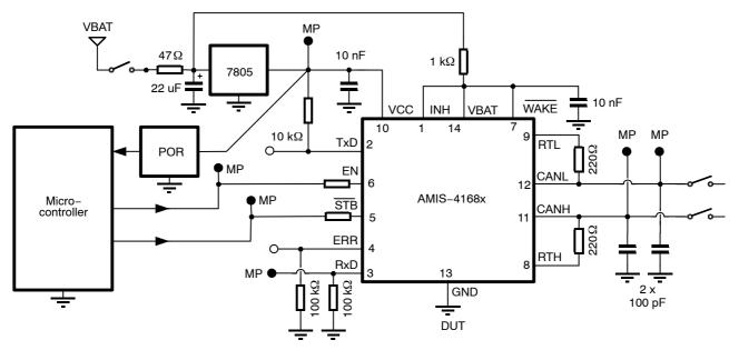
Figure 17. Measurement Set-up to Check the Initialization
