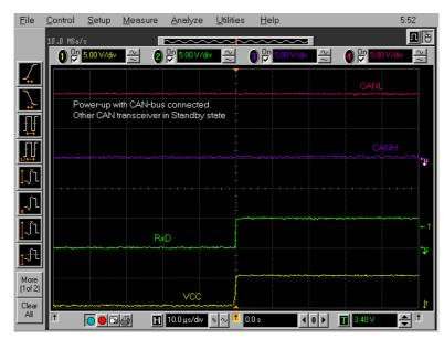
Figure 11. Power-up using set-up in Figure 10. The CAN-bus is in a permanent recessing state (CANL = VBAT) with the buskeeper in stand-by state. RxD becomes high after power-up of VCC.
