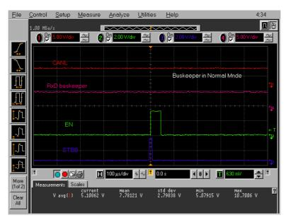
Figure 21. Buskeeper in stand-by mode. CANL termination switched from Vbat to Vcc for a short while (1.2 Tbits). No influence seen on RxD\_buskeeper.
