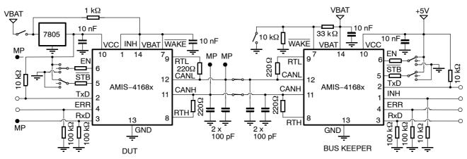
Figure 12. Measurement set–up: buskeeper in normal mode: EN = STBB = 1. For DUT EN = floating (internally pulled down) and STBB = 1.
