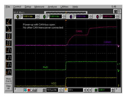
Figure 15. Power-up using set-up in Figure 14. The CAN-bus is open. RxD becomes high after power-up of VCC.
