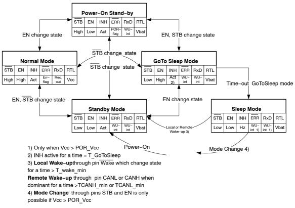
Figure 3. State Diagram Low Power Modes
