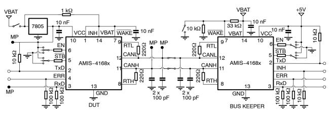
Figure 10. Measurement Set-up: Buskeeper in Stand-by State: EN = STBB = 0
