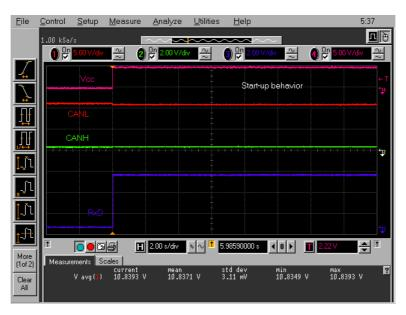
Figure 24. The CANL termination switched from Vbat to Vcc is not observable on a bigger time scale.
