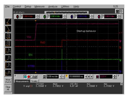
Figure 18. Start-up Behavior using the Proposed Sequence from Table 1
