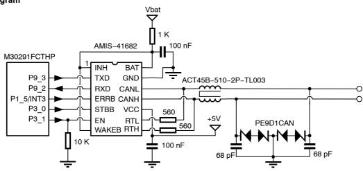
Figure 1. Application Diagram CANLSFT
