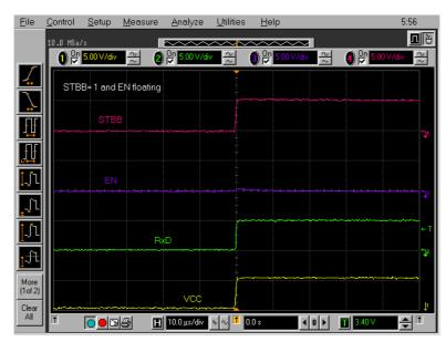
Figure 13. Power-up using set-up in Figure 12. The CAN-bus is in a permanent recessive state (CANL = VCC) with the buskeeper in normal mode.
