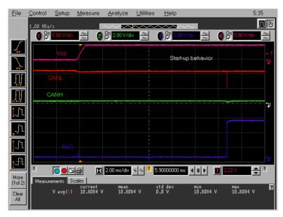
Figure 23. CANL termination switched from Vbat to Vcc for a short while (1.2 Tbit). No influence seen CANH. RxD switches high after the POR time-out.
