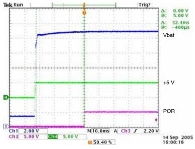
Figure 2. POR of the Microcontroller
