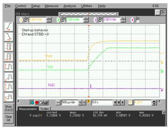
Figure 16. RxD stays low under specific conditions for Vcc and Vbat rise times and delay.
