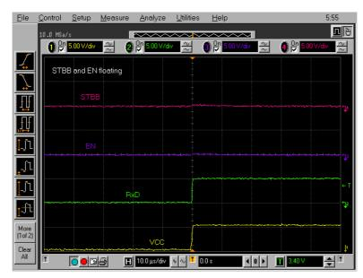
Figure 9. Power-up using set-up in Figure 7. Both STBB as EN are kept floating. The internal pull down resistors are keeping both levels low, also, during the rising edge of VCC. RxD becomes high after power-up of VCC.
