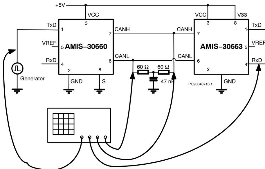
Figure 1. Measurement Setup
