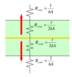
Figure 10. Spreader Plane Centered in Board
