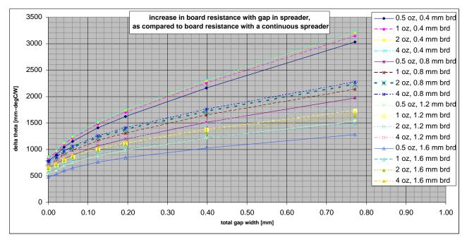
Figure 14. Increase in Board Thermal Resistance Due to Discontinuous Heat Spreader
