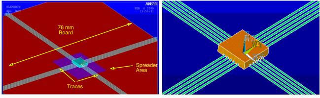
Figure 1. Spreader Area Centered Around QFN shown through transparent board
