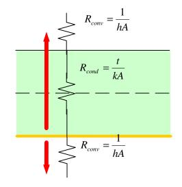
Figure 11. Spreader Plane on Surface of Board
