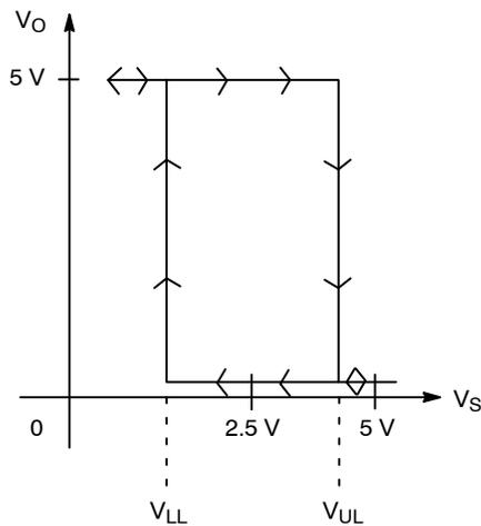
Figure 14. Transfer Characteristic
