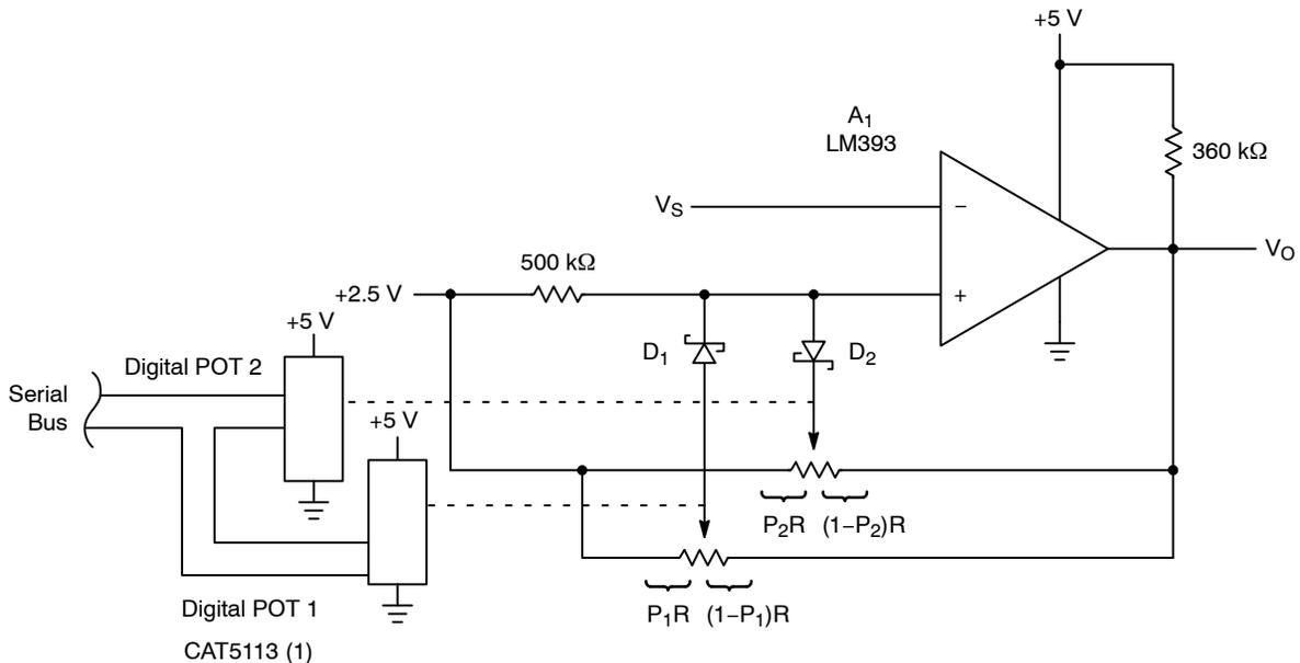
Figure 15. Schmitt Trigger with Independently Programmable Limits
