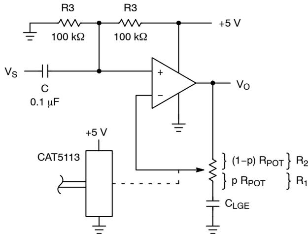
**Figure 2. Programmable Voltage Amplifier**
