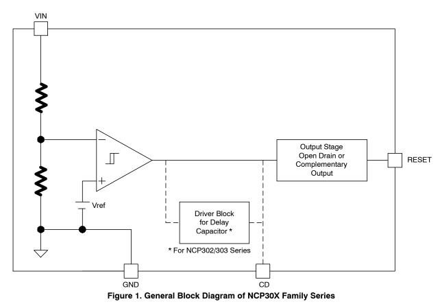
The Figure 1 shows the basic block diagram of NCP30X supervisory family series. It features a highly accurate undervoltage detector with hysteresis. Some parts also feature an externally programmable time delay generator by adding a delay capacitor at the CD pin. This combination of features prevents the system from erratic reset operation.
