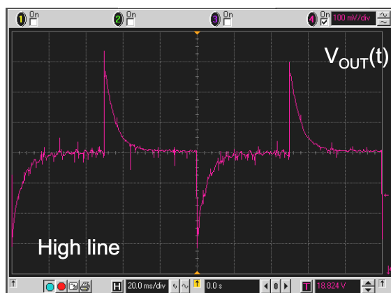
Figure 15. The Transient Response at Low Line and High Line Are Almost Identical and Do Not Show Signs of Instabilities
