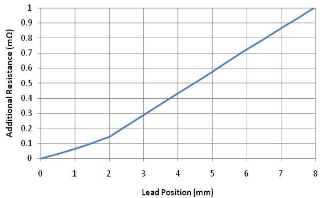
Figure 3. Added Lead Resistance for TO-220FP (mΩ)
