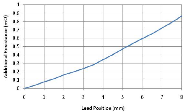
Figure 2. Added Lead Resistance for TO-220AB (mΩ)
