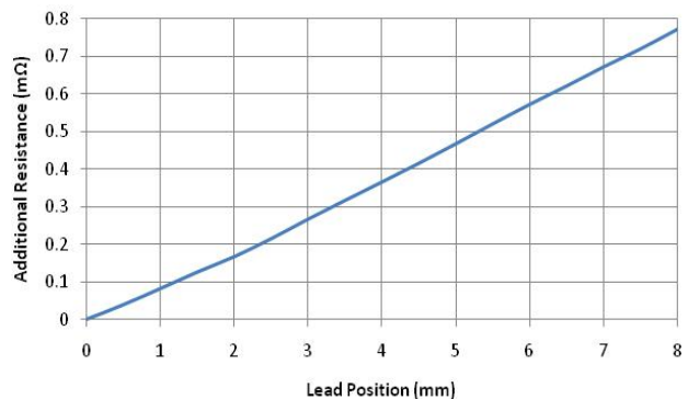
Figure 4. Added Lead Resistance for IPAK (mΩ)
