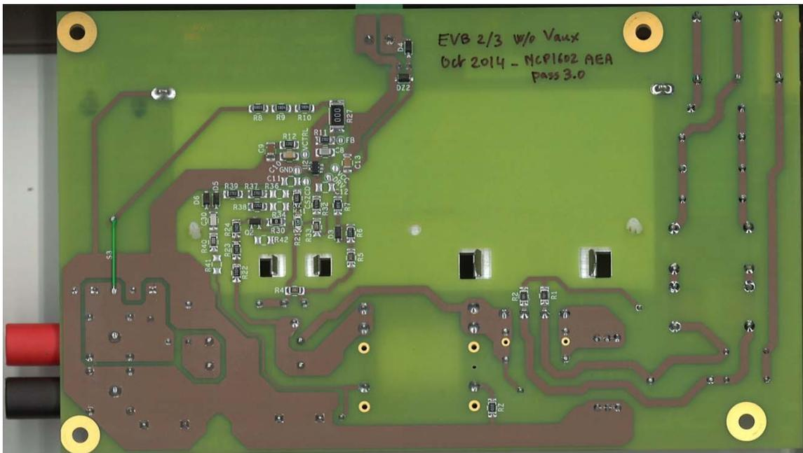
Figure 10. NCP1602 Low Profile Evaluation Board Bottom View Showing the Control Circuitry
