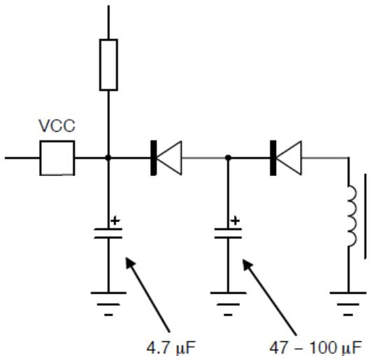
The 47µF capacitor does not load the Vcc terminal during start up thus assuring a fast start. After the converter starts switching, the 47µF capacitor provides a large energy storage element to keep the Vcc in the active region for a minimum of 50ms (the brown out detect period).
