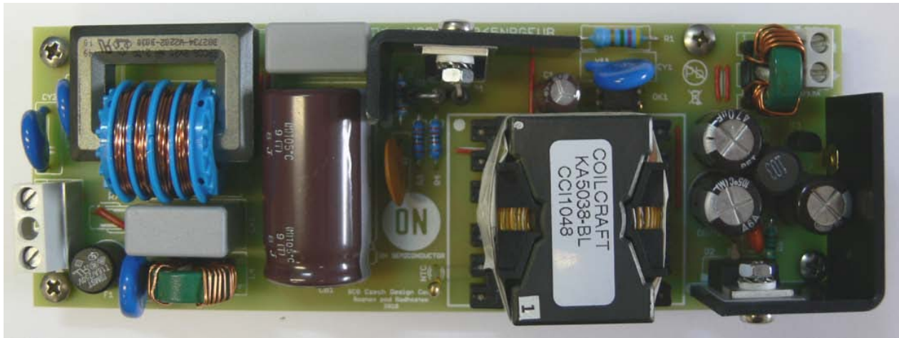
Figure 26. Photograph of the Designed Prototype (Real Dimensions are 146.6 x 50.8 mm)
