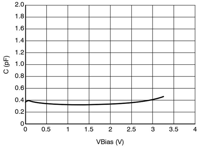
Figure 4. CV Characteristics
