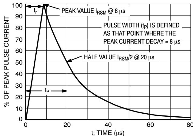
Figure 11. 8 X 20  $\mu$ s Pulse Waveform
