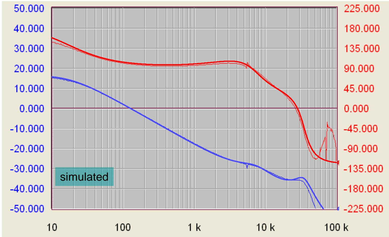
CCM operation,  $R_{load} = 6.3 \Omega$
