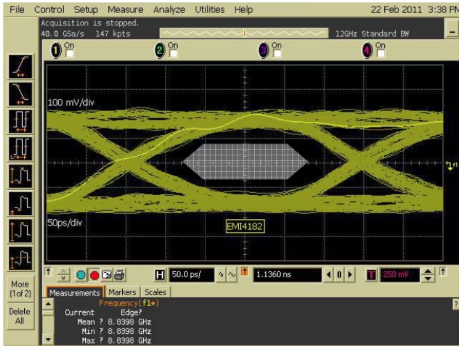
Figure 10. Signal Integrity Demonstration of Si CMF in HDMI 1.4 Environment
