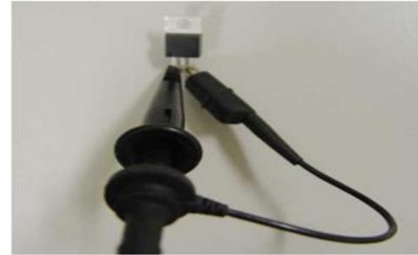
Probes are circuits composed of distributed R,L, and C for AC signals. → A total probe impedance varies with switching frequency.
