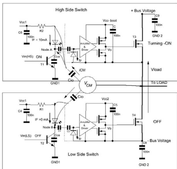
**Figure 10. Positive  $dv/dt$  - High-Side Switch Turning ON**
