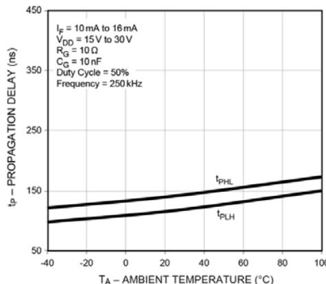
Figure 6. Propagation Delay vs.  $T_A$
