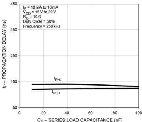
Figure 2. Propagation Delay vs. Series Load Capacitance
