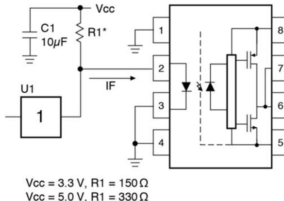
**Figure 11. FOD3182 with Shunt LED Drive**
