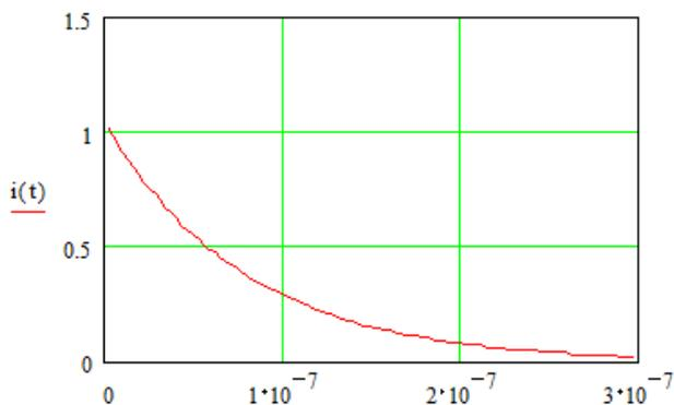
Figure 15. FOD3120 Output Current
