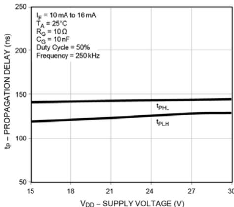
Figure 5. Propagation Delay vs. Supply Voltage
