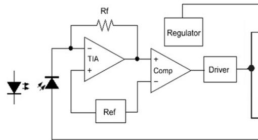
Figure 1. FOD31xx Block Diagram
