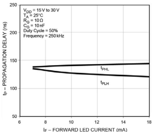
Figure 3. Propagation Delay vs. LED Forward Current
