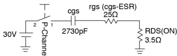
**Figure 13. Equivalent Circuit FOD3120 – MOSFET Interface**
