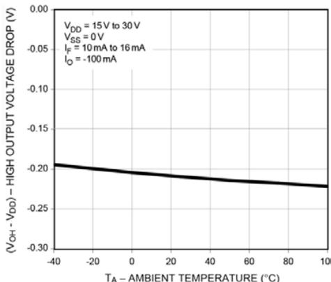
Figure 7. Output High Voltage Drop vs.  $T_A$
