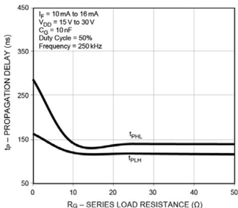
Figure 4. Propagation Delay vs. Series Load Resistance
