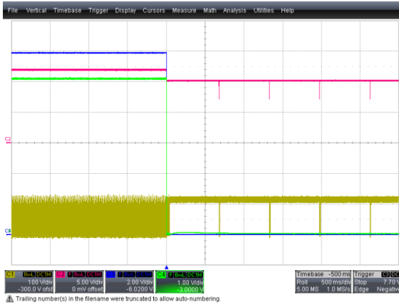
Figure 33. OLP Triggered, 12 V Output Short with 85 V AC , Full-Load, (CH1: V_{DS} (100 V/div), CH2: V_{CC} (5 V/div), CH3: 12 V_{OUT} (2 V/div), CH4: 5 V_{OUT} (1 V/div), Time: 500 ms/div)
