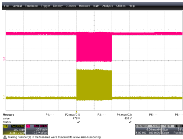
Figure 17. V_{DS}=451\text{ V} & V_{DIODE}=478\text{ V} , 12 V Output Short Condition, Full-Load Condition, 300\text{ V}_{AC} , (CH1: V_{DIODE} (200 V/div), CH2: V_{DS} (200 V/div), Time: 5 ms/div)
