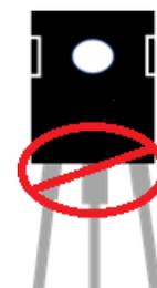
Figure 3. Sideways Bending May Cause Damage
