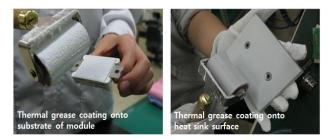
Figure 16. Applying Thermal Grease
