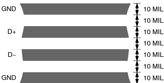
Figure 22. Arrangement of Signal Tracks
