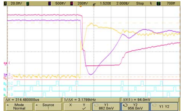
Figure 13. Typical Transient Response for Design Example Load Release 1-V O , 3-COMP, 4-TRDET, D 0 ~D 2 -PWM1~3
