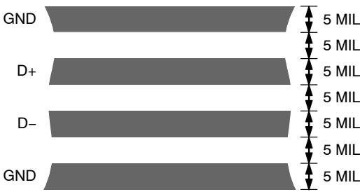
Figure 21. Typical Arrangement of Signal Tracks
